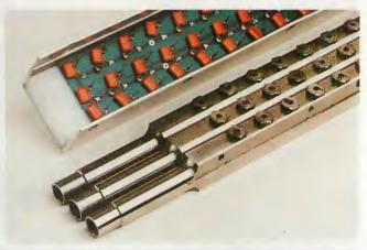
Resembling a "Robocop" movie weapon, Metal Storm's triple-barreled test gun is opened up to show its ignition ports. The cover plate (above) houses an array of electronic circuitry.
